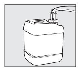
■ Insert the siphon tube into the container and screw on securely (observe the colour code).
